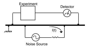
problem with reference frequency ground currents. In this illustration, the detector is measuring the signal relative to a ground far from the rest of the experiment. The experiment senses the detector signal plus the voltage due to the noise source's ground return current passing through the finite resistance of the ground between the experiment and the detector. The detector and the experiment are grounded at different places which, in this case, are at different potentials.
