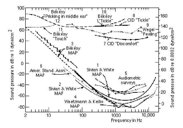
The so-called minimum audible pressure (MAP) (aka the reference pressure), is defined at f = 1 KHz and is:
