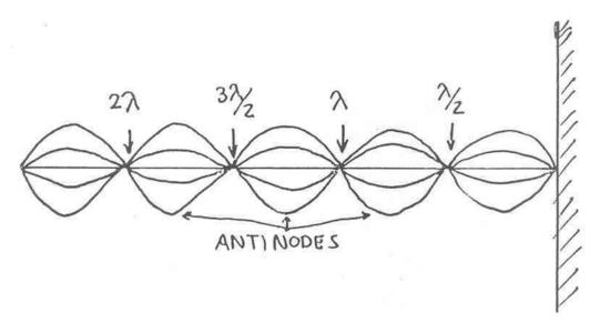
Anti-Nodes of transverse displacement occur at *x*-values along the string where  $sin(2\pi x/\lambda) = 1$ = *x*-positions along the string where transverse displacement is *maximum*: y(x,t) = A
