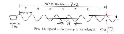
A = displacement amplitude of wave = max *displacement* from equilibrium position (meters, *m*)
