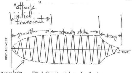
envelope Fig. 4. Growth and decay of a vibration.
