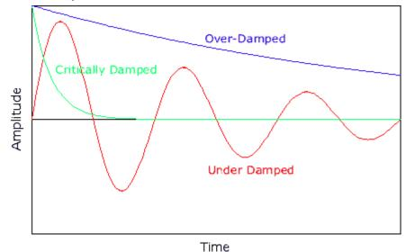
Note that damping processes that are operative in *all* musical instruments are in the *under-damped* regime (since by definition, to be musical, they *must* vibrate at frequencies > 0), typically with small amounts of damping, *i.e.*  $\gamma \ll \omega$ , such that:  $0 < \omega' = \sqrt{\omega^2 - \gamma^2} = \omega \sqrt{1 - (\gamma/\omega)^2} \le \omega$ .
