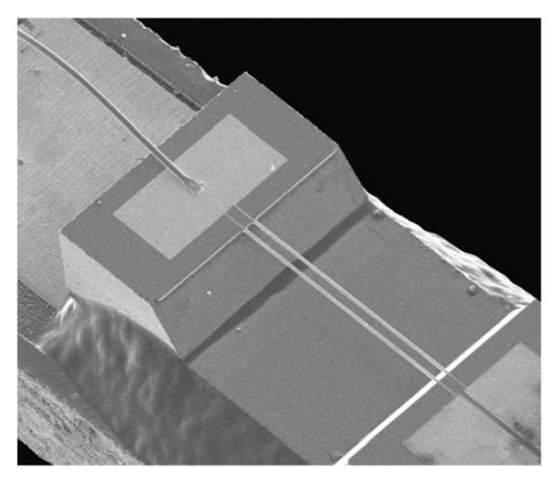
In a sound field  $\tilde{S}(\vec{r},t)$  the flow of air in the local vicinity of the two wires of the Microflown produces a small *differential* cooling of the two wires (this effect is similar, but not identical to the principle of how a so-called hot-wire anemometer works), as shown in the figure below:
