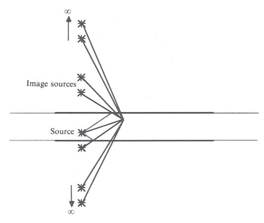
The pressure/particle velocity fields in proximity to the actual sound source inside the duct are determined largely by the image source(s) nearest to the actual sound source; the solution converges rapidly as the number of image sources is increased. However, accuracy in calculating the pressure / particle velocity fields far from the actual sound source (*i.e.* further down the duct,  $\Delta x \gg a$ ) requires increasingly larger numbers of image sources to be included.
