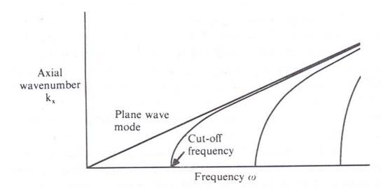
For a given (angular) frequency  $\omega$ , in general, the <u>total/net</u> complex pressure amplitude is a sum over <u>all</u> modes – the <u>allowed/propagating</u> individual complex pressure eigenmodes  $n \le n_{cutoff}$ , where  $n_{cutoff}$  is the <u>highest</u> eigenmode number n such that
