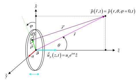
The surface of the plane circular piston oscillates harmonically back and forth along the  $\hat{z}$ -axis with complex velocity  $\vec{u}_p(z,t) = u_o e^{i\omega t} \hat{z}$ . What is the resulting complex pressure  $\tilde{p}(\vec{r},t) = \tilde{p}(r,\theta,\varphi=0,t)$  e.g. at an observation/listener point  $\vec{r} = (r,\theta,\varphi=0)$  lying in the x-z plane?
