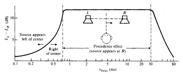
The horizontal axis is the time delay e.g. of a pulse to the LHS loudspeaker is delayed relative to the RHS loudspeaker. The vertical axis is the L–R difference in sound pressure level (SPL) due to the SPL of the LHS loudspeaker exceeding that from the RHS loudspeaker.
