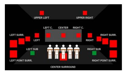
A 22.2 channel surround system has also been developed, for ultra-high definition television, which uses 24 speakers, arranged in 3 layers – a middle layer of 10 speakers, and upper layer of 9 speakers, a lower layer of 3 speakers and 2 subwoofers.
