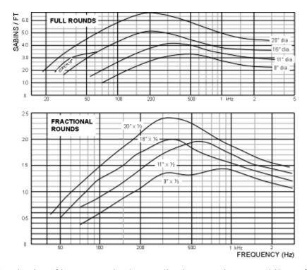
Note that the physics of bass traps also has applications e.g. in automobile muffler design!
