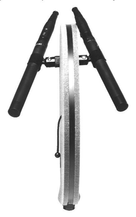
The specific arrangement of microphones used for stereophonic recording of sound/music is always a matter of taste – "beauty is in the ear of the beholder". For some people, the coincident microphone techniques sound dry and/or analytical – i.e. "too correct". However, a sensation of spaciousness can be created e.g. by introducing some signal delay between the two microphones, or by using spaced microphone pairs.
