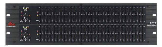
The use of a 31-band graphics equalizer – with 1/3 octave/band can significantly help in leveling out resonances {as well as anti-resonances/dips}in a room's acoustics, as shown schematically in the figure below:
