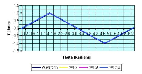
Fourier Construction of a Triangle Wave
