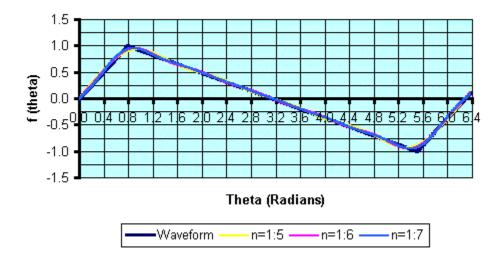
Again, adding on higher harmonics to the lower-order harmonics associated with the sawtooth wave makes for only small visual changes in the overall waveform - primarily, just the peak(s) sharpen as the higher harmonics are added.
