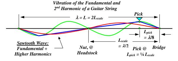
As can be seen from the figure, this picking location is *not* at the anti-node of the fundamental. It *is*, however at the anti-node associated with the second harmonic, an octave above the fundamental. The picking location is *near to*, but not *on* the anti-node of the third harmonic (e.g. see diagram, 2<sup>nd</sup> figure below). As mentioned earlier, this picking location is at the *node* of the fourth harmonic, which is the physical reason why *it* is not
