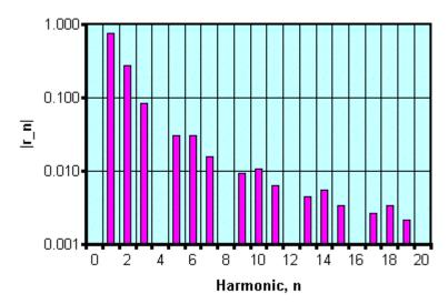
We can compare e.g. the relative strength of the third harmonic to the fundamental for the bipolar sawtooth wave to that for the third harmonic associated with the bipolar triangle wave. For the sawtooth wave,  $|r_3|/|r_1| = 11.1\%$ , while for the triangle wave, we also have  $|r_3|/|r_1| = 11.1\%$  - i.e. the same value of harmonic amplitude ratio! In fact the ratios  $|r_n|/|r_1|$  for  $\underline{all}$  odd-n harmonics are  $\underline{identical}$  for triangle vs. sawtooth waves!
