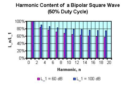
The following two figures show the "Fourier construction" of a periodic, bipolar, 50% duty-cycle unit-amplitude square wave. The waveforms in these figures were generated using truncated, finite-term version(s) of the Fourier series expansion for this waveform:
