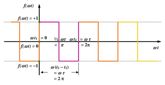
Since this waveform repeats indefinitely, then, without any loss of generality we can *arbitrarily* choose (i.e. re-define) the starting time,  $t_1$  of this waveform to be  $t_1 = 0$  seconds. Thus the ending time, for one period of this waveform is  $t_2 = \tau$  seconds. Then  $\theta_1 = \omega t_1 = 0$ , and  $\theta_2 = \omega t_2 = \omega \tau = 2\pi f \tau = 2\pi / \tau * \tau = 2\pi$ , since  $f = 1/\tau$ .
