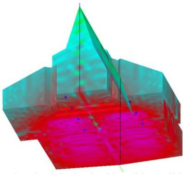
The above figure shows the solution. By using eight small, but very high quality speakers, mounted to, and partially hidden by the overhead beams, acoustical engineers were able to achieve excellent direct coverage of the congregation, putting very little acoustic energy on the walls. The red area is where the majority of the acoustic energy was directed, and as you can see, very little reached the walls.
