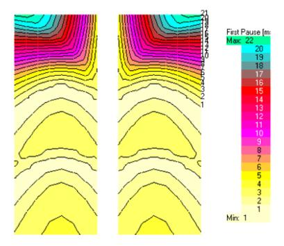
The above figure shows a color-coded contour map of the arrival time gap between the first and the second pulse in milliseconds. In other words, this figure shows the arrival time differential between the first of two adjacent sources. This is another way of looking at a sound systems predicted performance before any equipment is purchased. This same calculation in another design would help in the decision to utilize a stereo system.
