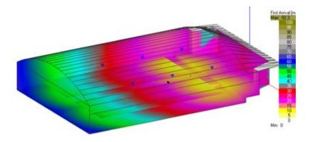
When using time-delayed speakers, as in this building, alignment of first arrivals from all the speakers is critical to maintain localization. The even flow of color indicates that the timing of the system is correct.
