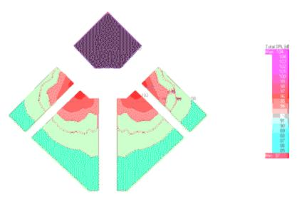
One important calculation EASE does is predicting maximum SPL (Sound Pressure Level). This image predicts the level to be between 98 and 103 dB at 1000 Hz. This would equate out to a system capable of 111 dB. Yes, 111 dB is really loud but since we would like to see no less than 6 dB and preferably 10 dB of dynamic headroom, this design satisfies that need, without paying for more acoustic output than necessary.
