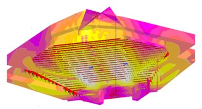
After completing the creation of the building in the computer, one can to run complex computations like the color-coded SPL map shown above.
