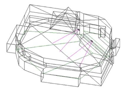
This is the beginning of a design using EASE. One builds a virtual room in the computer, entering geometrical data for the room point by point, then connect the dots. When complete, the virtual room is a wire frame drawing. Then every surface is defined in the computer. The computer needs to know what is on the surface and whether or not it is an audience/listening area. Once the data entry is complete, the computer with EASE software is used to perform complex audio calculations.
