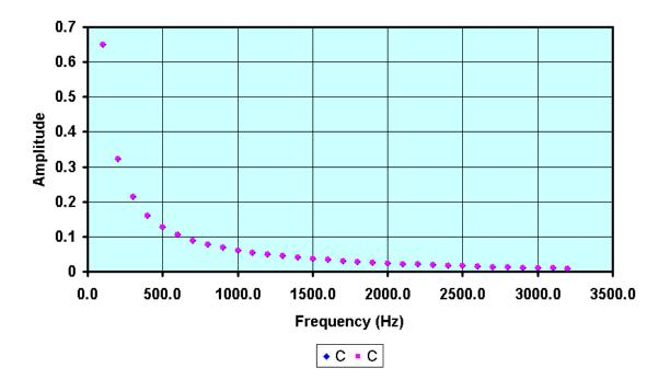
Harmonic Amplitudes for Second: D & C (Frequency Ratio 9:8) Sawtooth Waveforms, fo = 100 Hz, First 32 Harmonics
