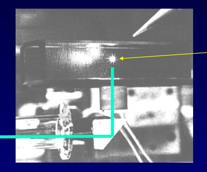
Glass bead 'floating' on a laser beam!
