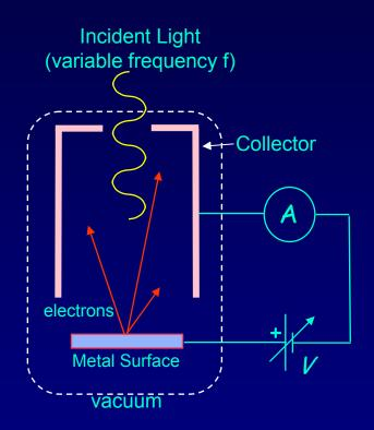
Bias the collector with a negative voltage to repel ejected electrons.
