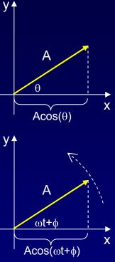
It is conventional to draw one phasor horizontal. Because the phasors are rotating, this merely means we are looking at them at a particular time.
