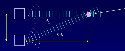
The two waves at this point are "out of phase". Their phase difference  $\phi$  depends on the path difference  $\delta \equiv r_2 - r_1$ .
