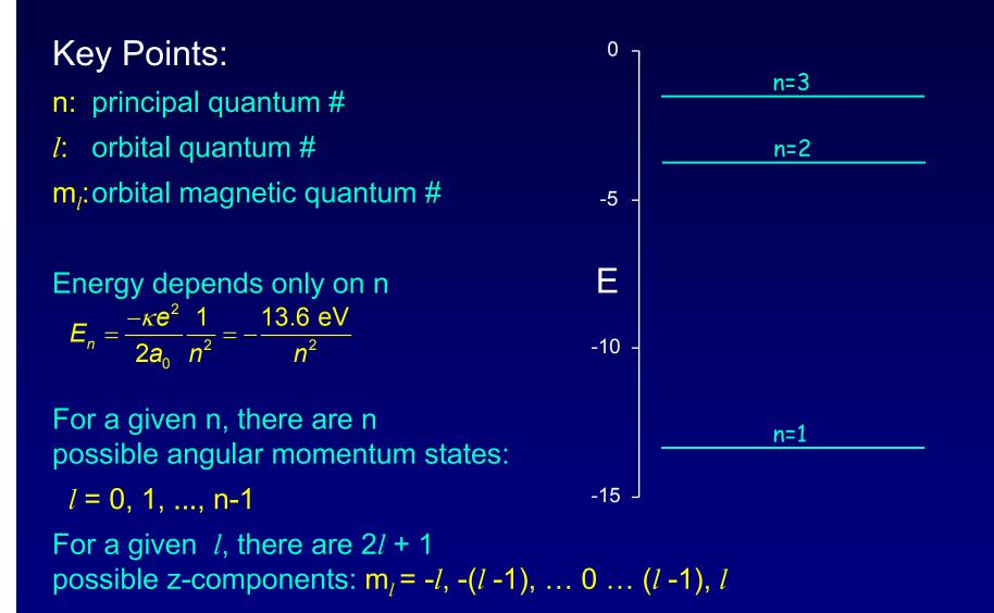
Therefore, a level with quantum number n has n<sup>2</sup> degenerate states.
