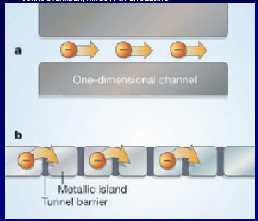
Electrons that successfully tunnel through the 50 junctions are detected using a fast single-electron transistor (SET).
