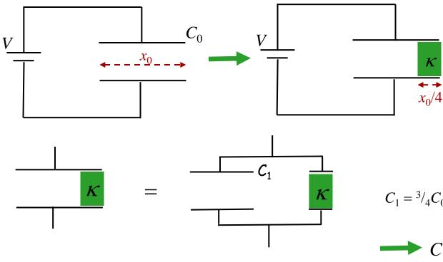
An air-gap capacitor, having capacitance  $C_0$  and width  $x_0$  is connected to a battery of voltage V.
