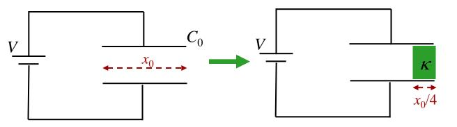
An air-gap capacitor, having capacitance  $C_0$  and width  $x_0$  is connected to a battery of voltage V.
