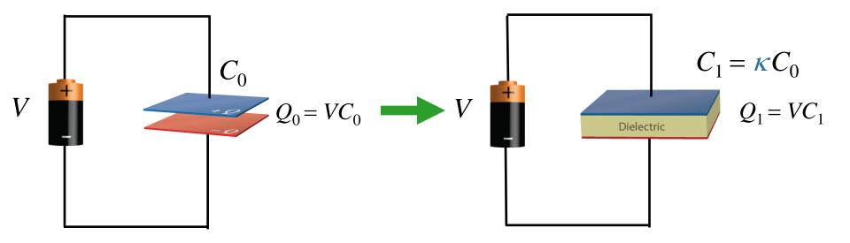
By adding a dielectric you are just making a new capacitor with larger capacitance (factor of *K*)
