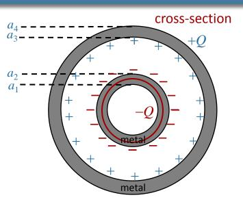
A capacitor is constructed from two conducting cylindrical shells of radii  $a_1$ ,  $a_2$ ,  $a_3$ , and  $a_4$  and length  $L(L >> a_i)$ .
