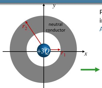
Point charge +3Q at center of neutral conducting shell of inner radius  $r_1$  and outer radius  $r_2$ .
