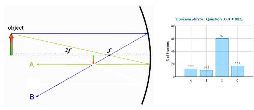
The diagram above shows two light rays reflected off a concave mirror. The image is
