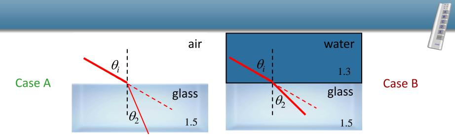
In Case A light in air heads toward a piece of glass with incident angle  $\theta_i$ In Case B, light in water heads toward a piece of glass at the same angle.
