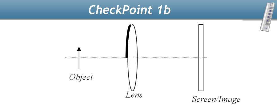
A converging lens is used to project the image of an arrow onto a screen as shown above
