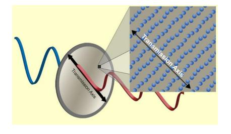
The molecular structure of a polarizer causes the component of the *E* field perpendicular to the Transmission Axis to be absorbed.
