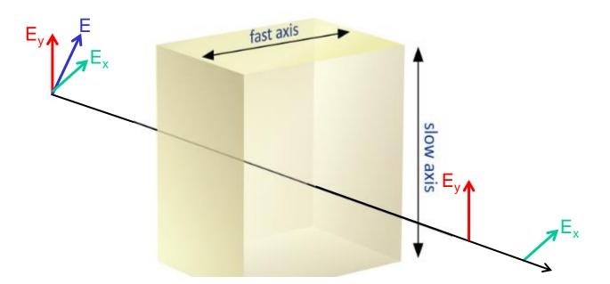
A linearly polarized EM wave is incident on a quarter-wave plate as shown above. The resulting wave is
