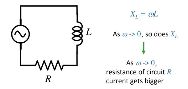
For what driving frequency  $\omega$  of the generator will the current through the resistor be largest
