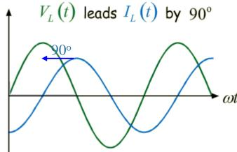
where  $X_L = \omega L$ is like the "resistance" of the inductor  $X_L$  depends on  $\omega$
