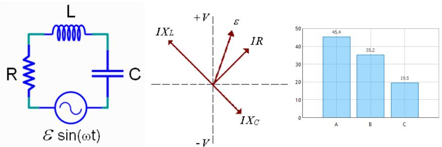
The vertical axis of the phasor diagram represents voltage. When the current through the circuit is maximum, what is the potential difference across the inductor?
