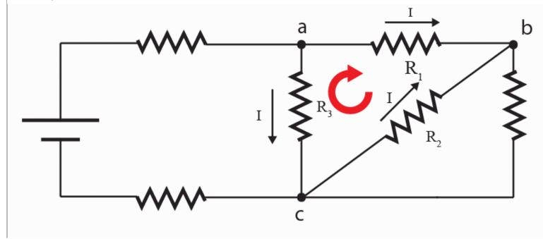
If we are to write Kirchoff's voltage equation for this loop in the clockwise direction starting from point a, what is the correct order of voltage gains/drops that we will encounter for resistors R1, R2 and R3?
