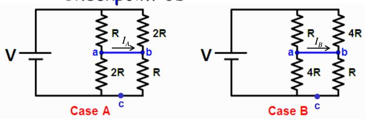
which case is the current flowing in the blue wire connecting points a and b the largest?
