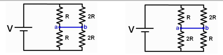
What is the same? Current flowing in and out of the battery.
