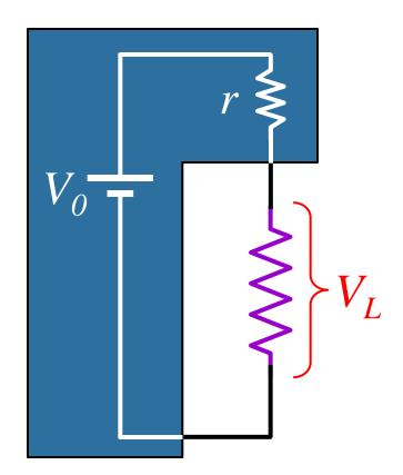
Usually can't supply too much current to the load without voltage "sagging"
