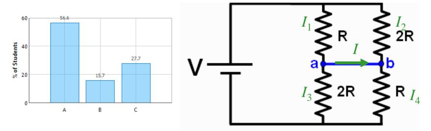
Which of the following best describes the current flowing in the blue wire connecting points **a** and **b**? **A.** Positive current flows from *a* to *b* **B.** Positive current flows from b to a
