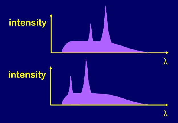
The top spectrum comes from a tube with a silver target (Ag, Z=47). What is the bottom target?
